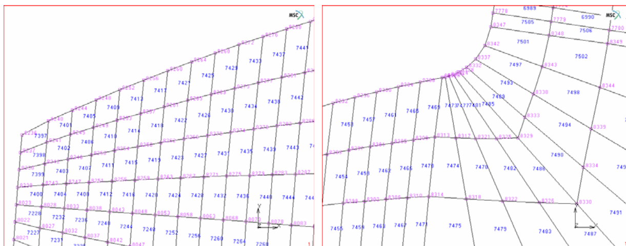
Figure 34: Gear numeration of node and elements: a) Detail of the tip of tooth 22; b) Detail of the right side fillet of tooth 22.
